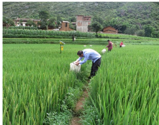
Figure 56: Weekly air sampling in collection boxes for methane content measurements.
